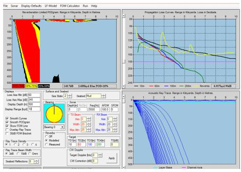
The Analysis Screen includes Reverberation Limited PODgram (shows Sonar Detection Range and Performance Prediction), Propogation Loss Curves Diagram, Displays Option, Surface and Seabed, Sonar and Target Modification Options and Acoustic Ray Trace.
