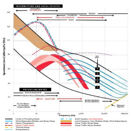
The Wenz Curve is use to determine Ambient Noise cause by various environmental factors.
