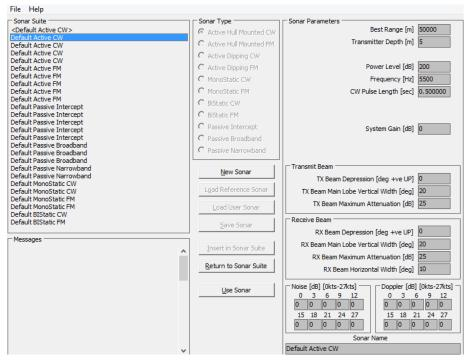
Sonar Editor for operator to fill according to the technical data of own ship sonar.
