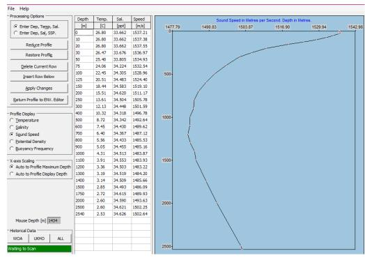
Profile Editor can be used to measure accurate Sound Velocity Profile using real time or in-situ sea temperature, salinity and/or depth data information.
